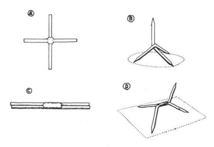
Two possible methods of making caltrops. Top: weld a cross, bend and sharpen. Bottom: weld side by side, bend and sharpen.
