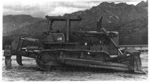
Bulldozer. Note the smoke stack (exhaust pipe).
