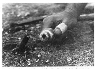
Note the "seat" created in the end of the driver (the  $^{1/4}$  inch nipple screwed into one of the reducers).
