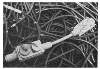
Seismic cable. Note cableheads.
