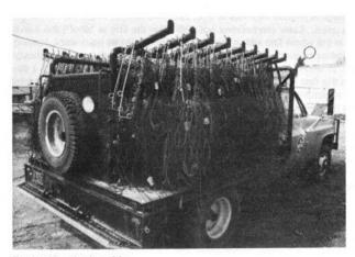
Truck with seismic cable.
