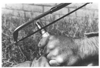
Finally, saw off the  $\frac{1}{4}$  inch nipple flush with the reducer. Your road spike driver is ready for use.
