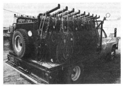
Truck with seismic cable.
