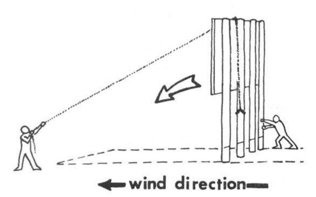
Tie the rope high up on a pole and throw the remainder over the top (you may have to weight the end with a rock). Make sure the rope is long enough to keep you out of the danger zone.
